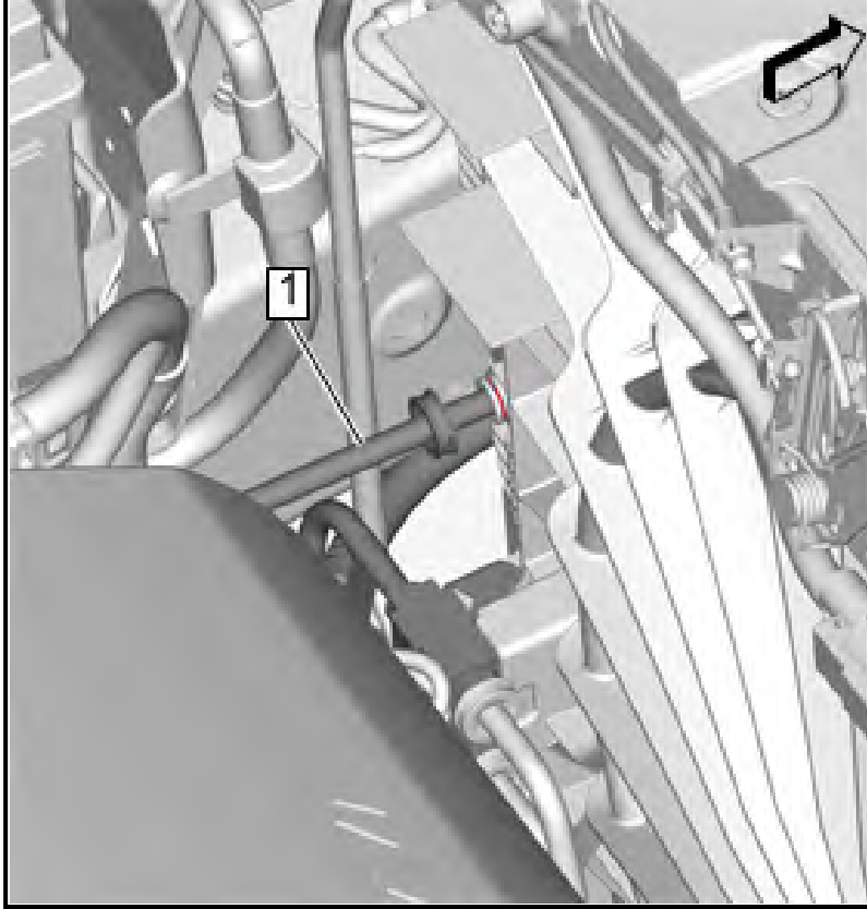
Transmission Fluid Cooler Thermal Bypass Valve (1) @ Radiator - Connect - Transmission Fluid Cooler Hose/Pipe Quick-Connect Fitting Disconnection and Connection
