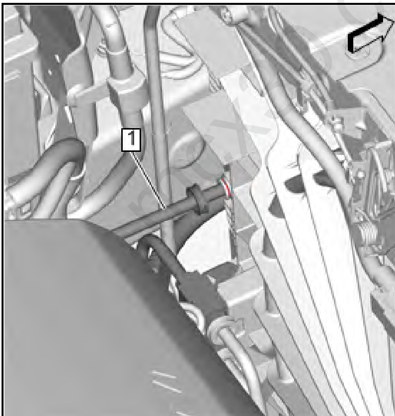
Transmission Fluid Cooler Thermal Bypass Valve (1) @ Radiator - Disconnect - Transmission Fluid Cooler Hose/Pipe Quick-Connect Fitting Disconnection and Connection
